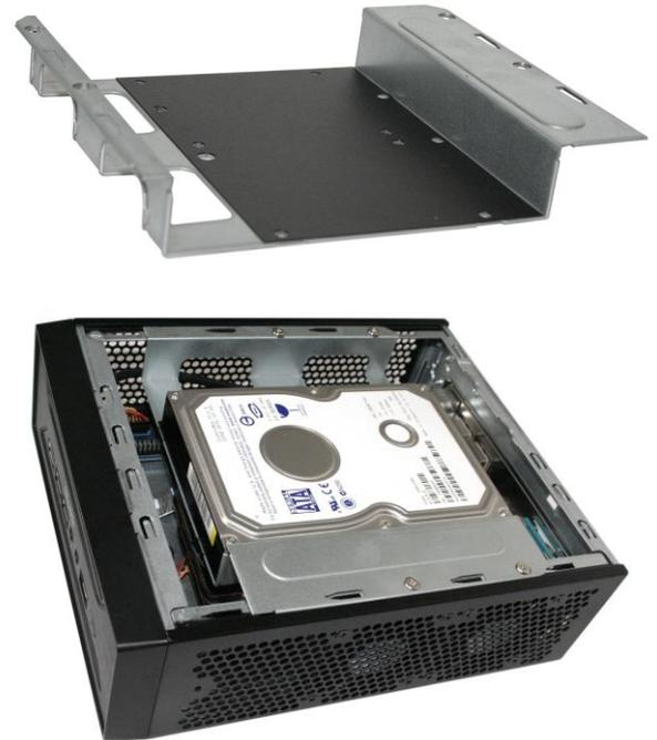
Shuttle Slim-PC Barebone (3 litres) with built-in Accessory PHD4 including 3.5" hard disk drive.
